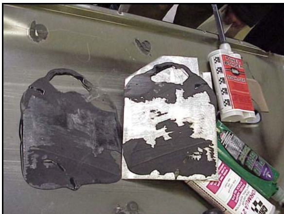
COHESIVE FAILURE EXHIBITED @ 60% ADHESIVE FAILURE EXHIBITED @ 40%
